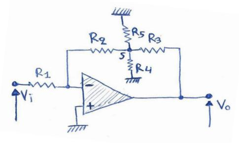
(b1: 1/2 points) Calculate the potential at point S (b2: 1 point) Calculate the closed loop gain Vo/Vi
