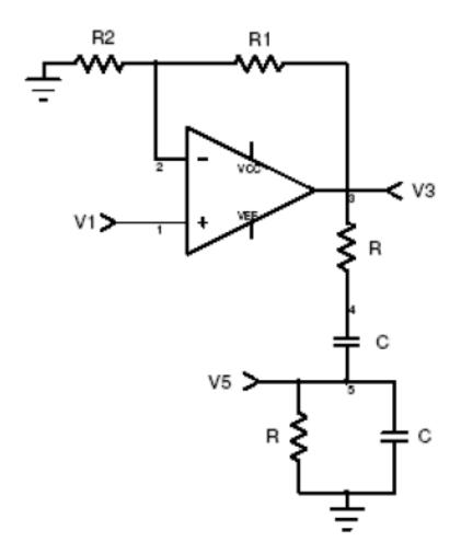
(a: 1/2 points) Calculate the transfer A = V(3) / V(1)
