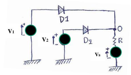
(a: 1/2 point) The diodes D1 and D2 are ideal with forward conduction voltage Vc=0.7 V. Explain briefly which diode conducts current, and justify your answer. Consider V1=4 V, V2=9 V, and Vs=2 V
