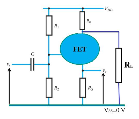
Show that the amplification ratio  $\upsilon_o / \upsilon_i$  of the small voltage variation at the input/output is given by:
