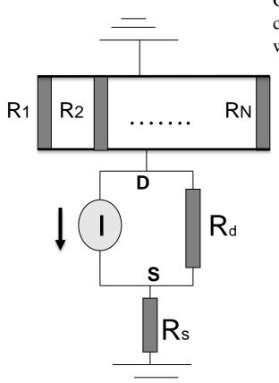
Consider the current source I in the circuit shown below to be parallel with a resistor Rd
