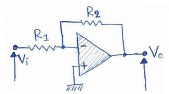
(a1: 1/2 points) Calculate the closed loop gain Vo/Vi (a2:: 1/2 points) Calculate the limit of Vo/Vi for an ideal opamp with  $A \rightarrow +\infty$
